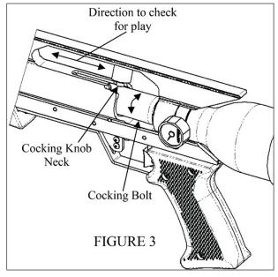
Step 2. Rotate the Cocking Bolt to either side of the gun. The Cocking Knob Neck has to clear the narrow channel in the frame, slipping into the widened area of the channel.
