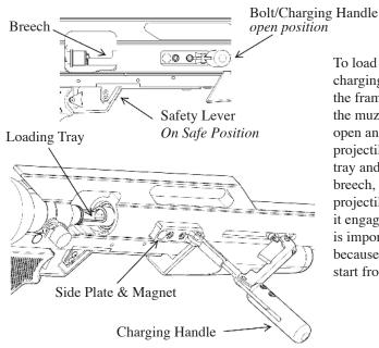
To load the rifle, pull the charging handle away from the frame and push it toward the muzzle until it cannot open any further. Place a projectile in the loading tray and push it into the breech, with your thumb or a projectile seating tool, until it engages the rifling. This is important for accuracy, because it makes each shot start from the same place.
