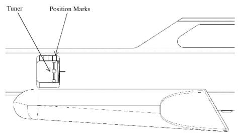
To increase tuner tension rotate it downwards, to decrease tension rotate it upwards. Increasing tension can help achieve higher velocities for light-weight projectiles.
