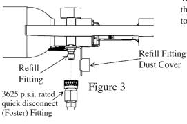
To refill your Spin-Loc Tank, attach the 3625 p.s.i. rated quick disconnect to the refill fitting. See FIGURE 3. ▲ WARNING: BEFORE LOADING YOUR AIRGUN, MAKE SURE THE SAFETY IS IN THE ON SAFE POSITION AND THE MUZZLE IS POINTED IN A SAFE DIRECTION.
