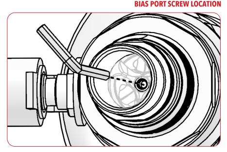
**Above:** The included 2mm hex key fits into the valve pin to access the Bias Port Screw. Turn counterclockwise to loosen, or clockwise to tighten. Secure to 3 inchpounds of torque.
